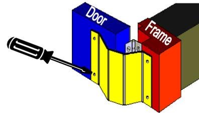
6. Peel off the protective tape from the other side of the door finger guard and repeat the procedure in 5. to attach it to the door.
