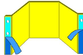
4. Peel off the protective tape from one side of the door finger guard.
