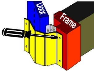
5. Line up the edge of the door finger guard to the guideline on the door-frame and press firmly in place.
