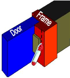
1. With the door shut and the measuring block vertical (20 mm width) draw a guideline on the door-frame.
