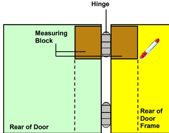
**Step 1:** With the door shut and the measuring block horizontal (30mm width) draw a guideline on the door frame.
