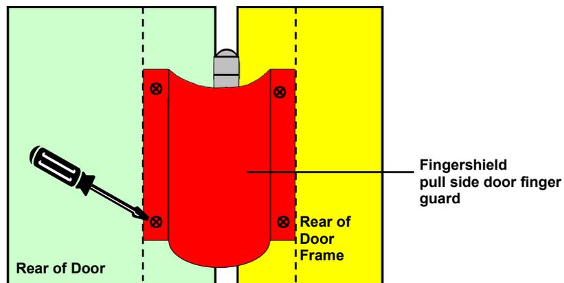
**Step 3:** Peel off the protective tape from one side of the door finger guard. Line up the edge of the door finger guard to the guideline on the door-frame and press firmly in place.
